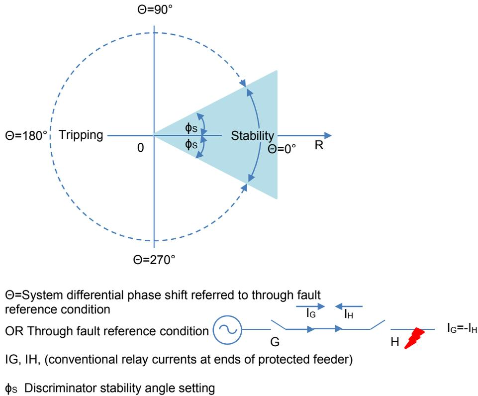
Figure 13. Polar diagram for phase comparison arrangement
