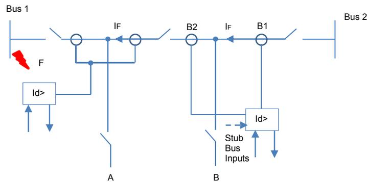
Figure 11. Breaker and a half switched substation arrangement
