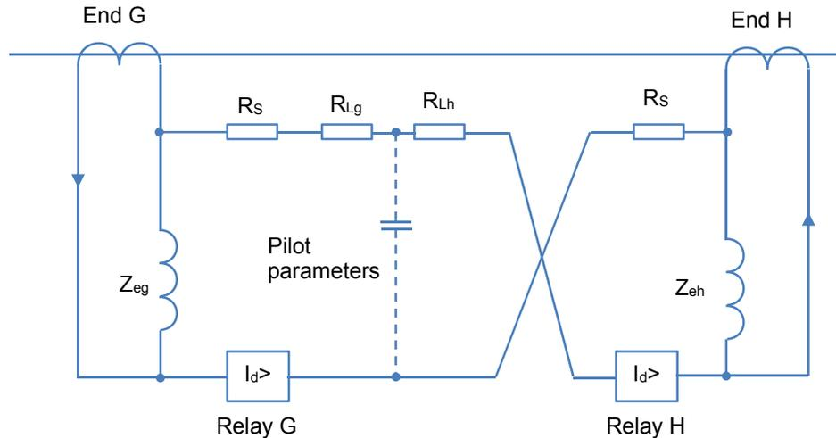
Figure 6. Equivalent circuit for balanced voltage system
