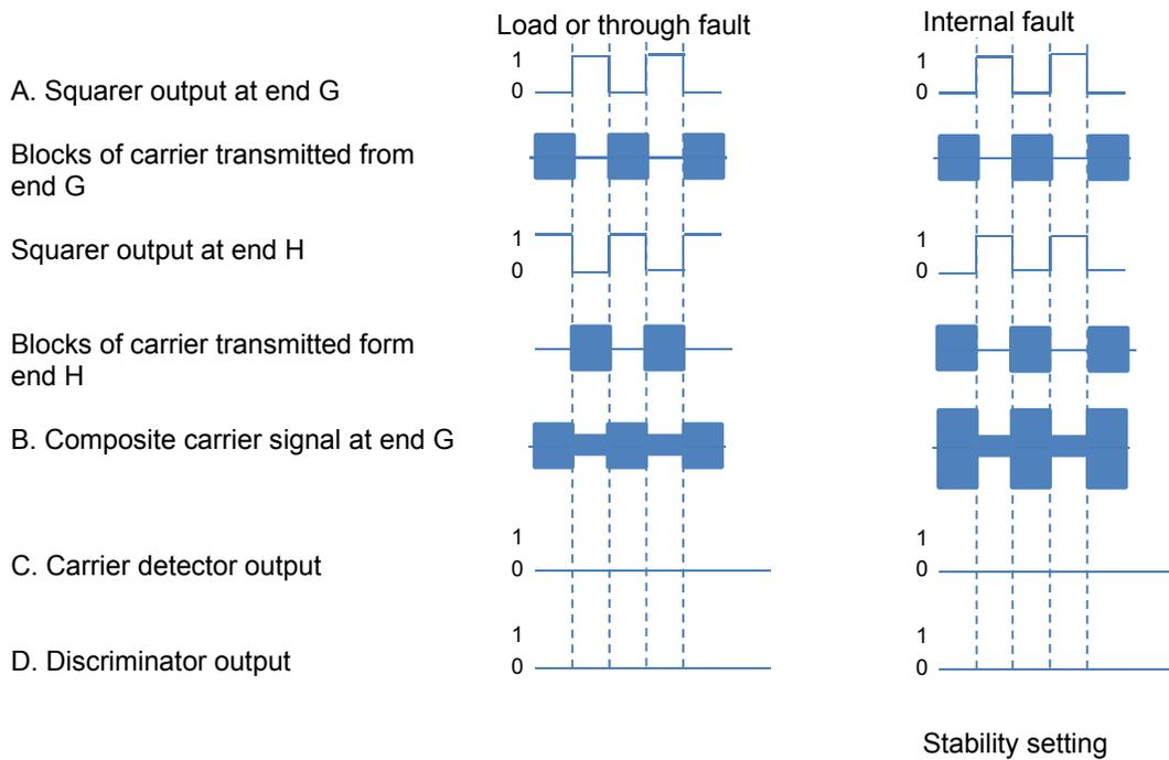
Figure 14. Basics of power line carrier phase comparison
