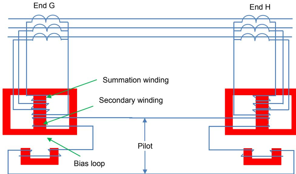
Figure 8. "Translay" biased electromechanical differential protection arrangement
